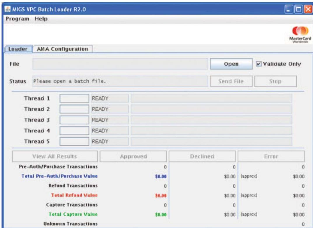
The main "Loader" screen is the interface through which the user will carry out the batch processing task. Notice that the "Batch File" field is currently blank, and that the "Load" button is disabled.
