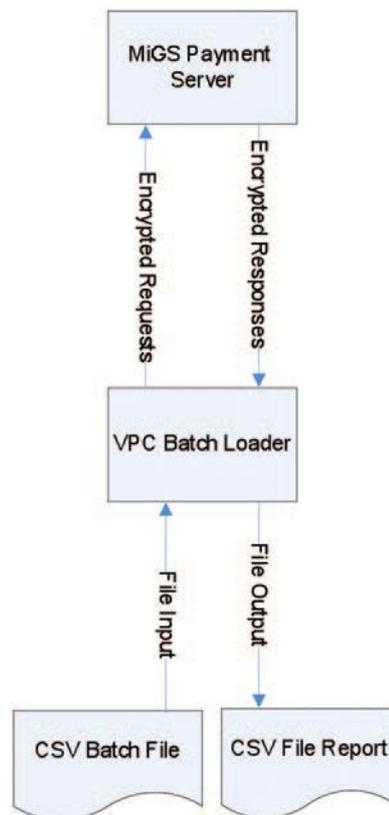
Communication between the Batch Loader and the Server
